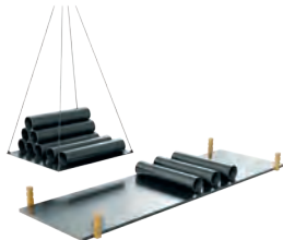
1 Transportation of Bare Pipe from Stockpile to Coating Plant
